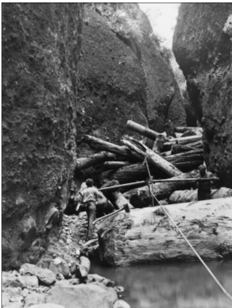
Freeing a jam of kauri logs with the aid of a 'bush devil', c 1900. Photographer Albert Percy Godber. From the Making New Zealand collection, photograph courtesy of the Alexander Turnbull Library (MNZ -1754-1/2)
